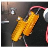
3. Screw both resistors on a clean grinded metal surface for heat dissipation. (When unscrewed, resistor temperature can rise up to 100 degres celcius.)
