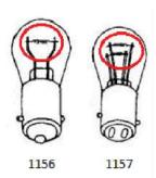
The bulb bases generally used for position lights, brakes, turn signals are as follows:
